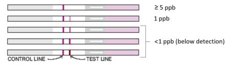
Alternately, test strips can also be interpreted using the AbraScan test strip reader (PN 475025), which provides objective determination of line intensities for consistent interpretation of results as well as a digital photographic record of all test strips.
