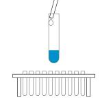
Add 500 μL of Color Reagent down the inside wall of each tube by using the technique described in Box 2.
