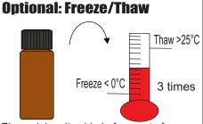
Place vial on its side in freezer to freeze and then thaw sample at room temperature. Repeat process two more times. Please refer to user's guide for more information.
